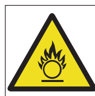
Ref. 385 Peligro Material comburente
