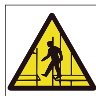
Ref. 317 Peligro andamio incompleto
